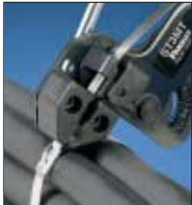
Hand operated tool with installer controlled tension and cut-off.
